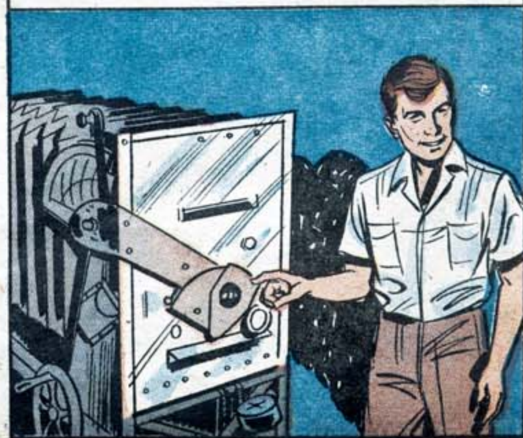
"THE 'CROPPED' PHOTO IS SENT TO THE ENGRAVING DEPARTMENT WHERE BIG CAMERAS REPHOTOGRAPH IT THROUGH GLASS PLATES WHICH HAVE THOUSANDS OF TINY CROSS LINES... THIS SCREEN-PLATE BREAKS THE PICTURE INTO THOUSANDS OF TINY DOTS PER SQUARE INCH."
